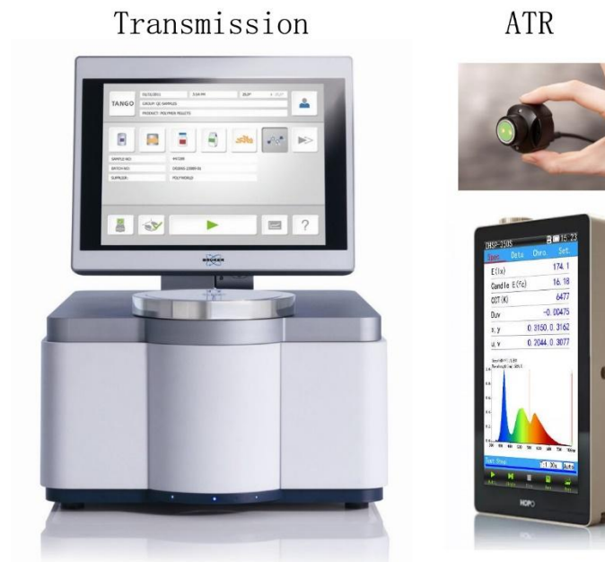
Fig. 6, The desktop NIR spectroscopy needs to prepare the sample into a compressor, the spectrals are collected after the transmission of NIR (left). The portable NIR spectrometer is based on the modern linear variety filter (LVF) and ATR technology, which can directly scan the same and the NIR spectrals can be analyzed locally and remotely.
